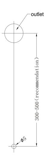
1.Drill a  $\phi$ 6mm hole at the outlet vertical downward position in the recommended range.
