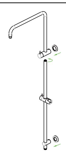
3.Screw shower rail into shower arm component. Tighten firmly. Push 2 back plates onto shower arm component and lower mounting pillar.
