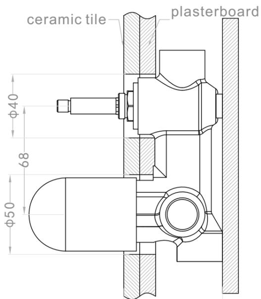
1. Fix body on noggin and ensure installation depth is 62-76mm from noggin to ceramic tile.
