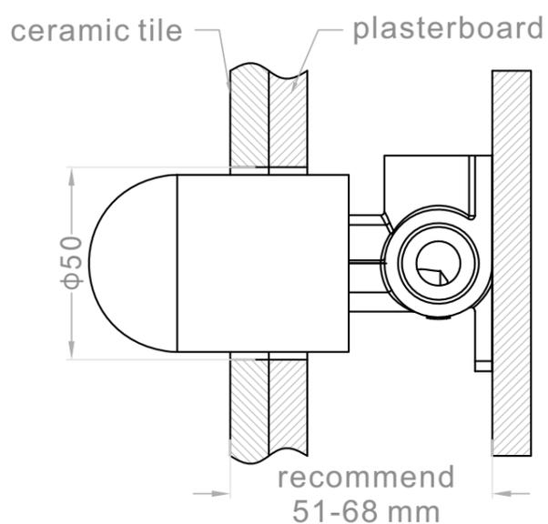
1. Fix body on noggin and ensure installation depth is 51-68mm from noggin to ceramic tile.
