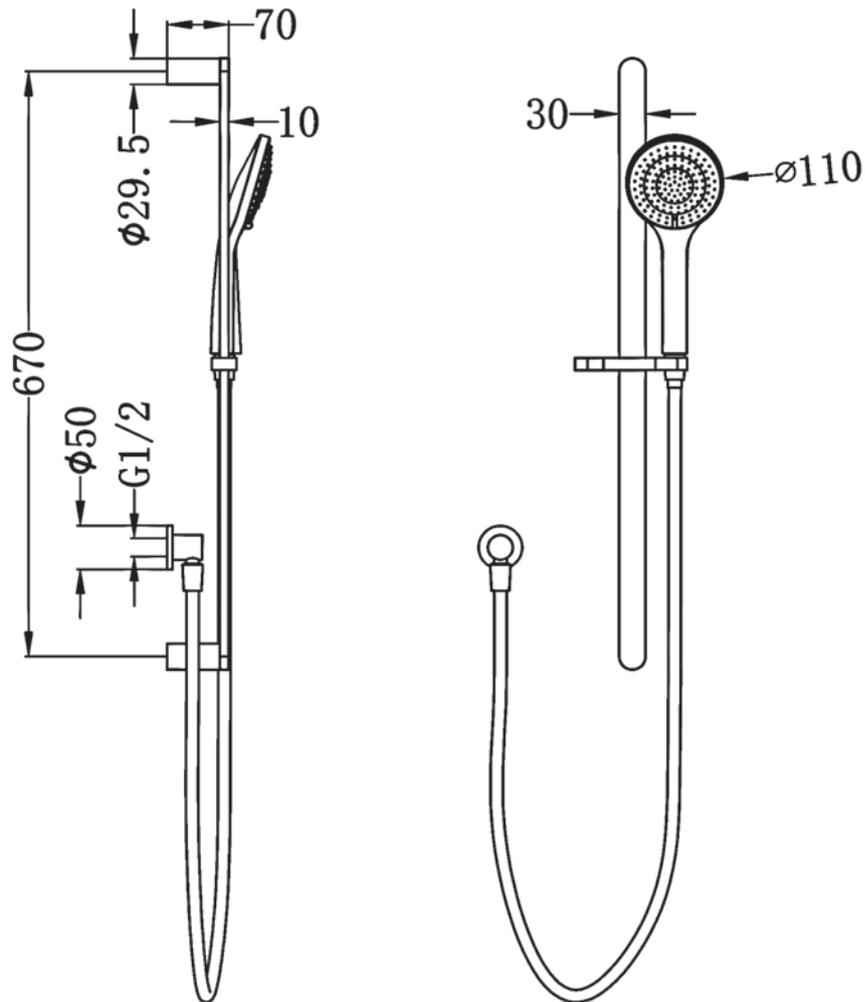
2. The inlet of the shower hose is connect to a wall elbow installed by the plumber at a suitable height.
