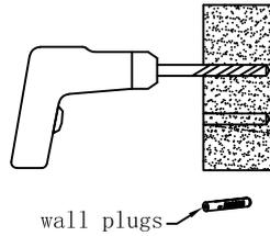
5. Drill pilot holes into wall stud approximately 60mm deep to suit mounting screws (and wall plugs if required).
