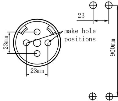
4. Locate wall studs, install into at least one stud. Place wall seal/mounting bracket on wall at correct height over centre of stud and mark hole positions on wall.
