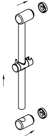
8. Slide the shower slider onto rail, then slide rail tubes into end brackets and push onto wall brackets, refer to above picture.
