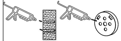
6. Apply small amount of silicon to mounting bracket and wall in and around the screw holes.
