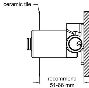
1. Fix body on nogging and ensure installation depth is 51-66mm from nogging to ceramic tile.
