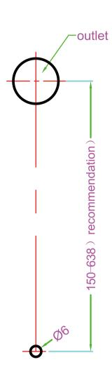
1.Drill a φ6mm hole at the outlet vertical downward position in the recommended range.
